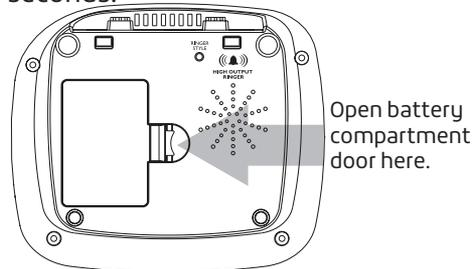
To install batteries in the base:
